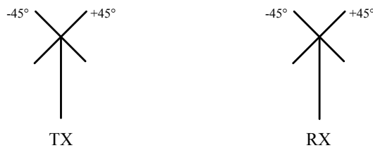
Figure 2.6: Illustration of a dual polarized antenna setup.
